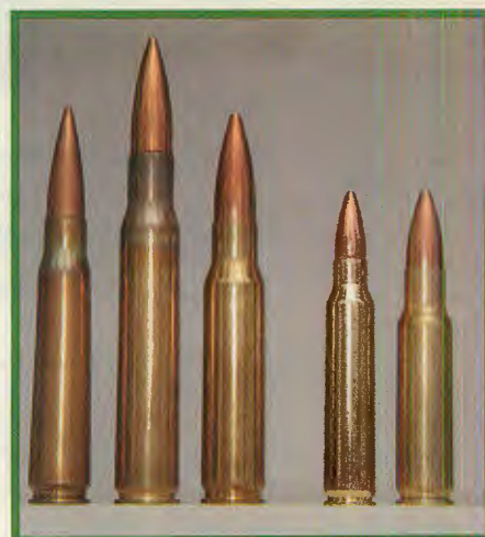
From the left are the .276 Pedersen, .30-06 (.30 M2), 7.62x51mm NATO, 5.56x45mm NATO and the 6.8mm Rem. SPC. Except for size, the characteristics of the 80-year old .276 and 6.8mm are surprisingly similar.
