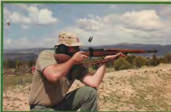
As Sgt. Joe Scott fires the last round of .308 from the Krieger Match Grade M1, the rifle automatically ejects the empty clip with the characteristic "ping."
