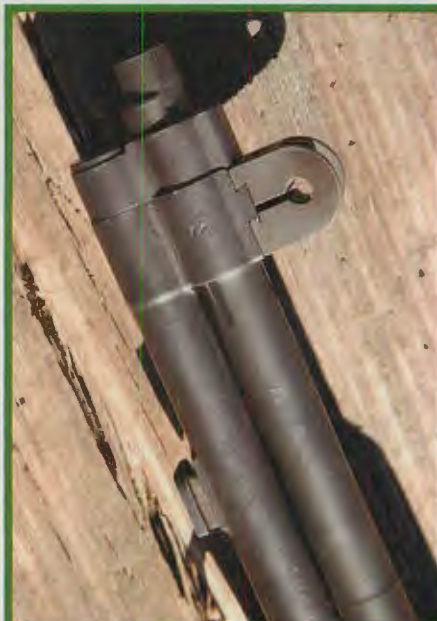
National Match M1 rifles are stamped or engraved with the letters NM on the left side of the barrel. The first NM Garands also were stamped with a star, as seen here.
